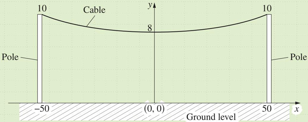
The height of the cable is given by  $y = c(e^{kx} + e^{-kx})$  where  $c$  and  $k$  are positive constants.
