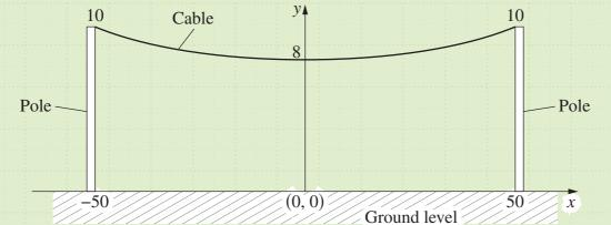
The height of the cable is given by  $y = c(e^{kx} + e^{-kx})$  where c and k are positive constants.
